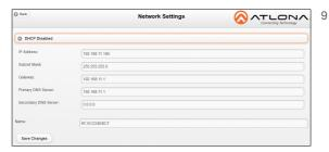
Type in the IP details to match the network details of the Gateway. e.g. If the Velocity gateway is located at the IP of 192.168.12.15, then the VCC should be set to an IP within the 192.168.12.XXX range that has not already been used.
