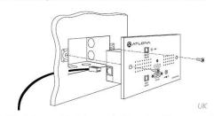
The UK wall plate screws will be the longer than the US screws. Thread the screws through the two holes in the UK wall plate and into the back box (as shown above).
