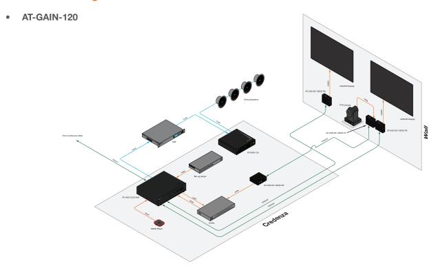
• AT-GAIN-120 with AT-GAIN-NET networked audio card
