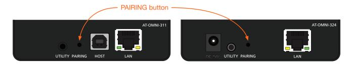
3. Release the **PAIRING** button after approximately 10 seconds. The **LINK** LED indicator will begin flashing. Pairing mode is now active on the OmniStream 311.
