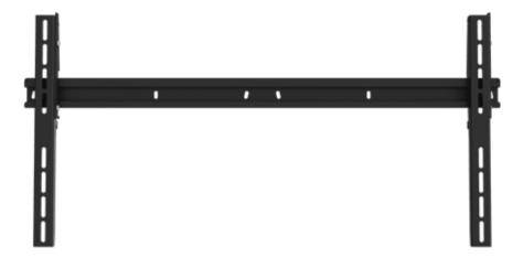
A universal wall bracket for screens of dimension up to 55". Simple to mount, the hole patterns have been designed such that the bracket fits exactly between two wall studs. Can be tilted in steps, and designed to be locked by a locking pin or padlock for improved personal safety and security from theft. Suitable for Vesa hole patterns with maximum dimensions  $800 \times 400 \text{ mm}$  and minimum dimensions  $100 \times 100 \text{ mm}$ .
